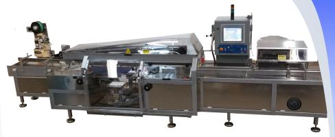
Bagger: Straight or "J" style cross-feed discharge conveyor
